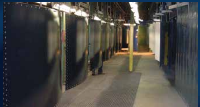
▲ Glass-fused-to-steel panels on the production line.
